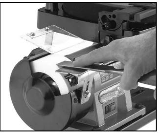
Figure 8. Grinding on dry wheel.
